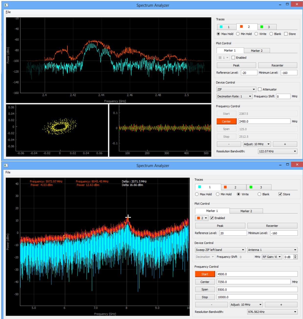
`rtsa-gui` is a cross-platform GUI application built with the Qt toolkit and PySideProject bindings for Python.
